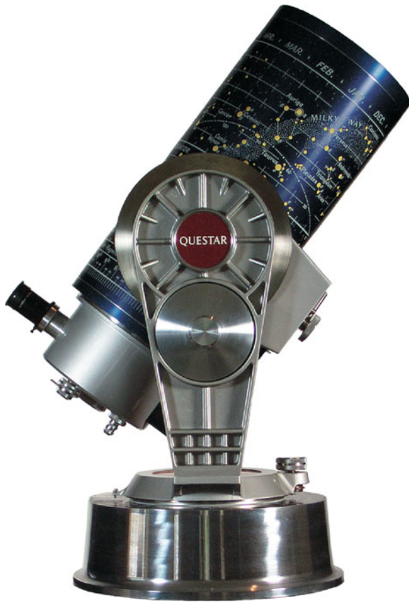
Fig. 6.3 The standard Questar’s big brother—a 7-in. Maksutov-Cassegrain. At double the aperture, it has twice the resolution and four times the light-grasp of the smaller instrument, but also much greater cost and weight. Courtesy of Questar Corporation
