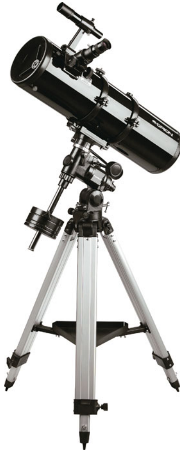
Fig. 5.2 Orion's AstroView classical 6-in. Newtonian reflector, shown here on a German equatorial mount. The traditional focal ratio for a 6-in. long-preferred by telescope makers and observers was (and for many still is) f/8 . But in a bid to make telescopes more compact and portable, shorter ones have appeared on today's market—as in this case, which is an f/5 system. Courtesy of Orion Telescopes & Binoculars
