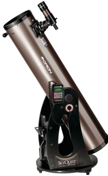
Fig. 5.4 Orion’s line of SkyQuest IntelliScope Dobsonian reflectors feature Push–Pull-To computerized technology to locate objects. The hand controller (seen here on the 8-in. model) indicates the location of a desired object while the observer moves the telescope until a “null” reading appears on the LCD display. Courtesy of Orion Telescopes & Binoculars
