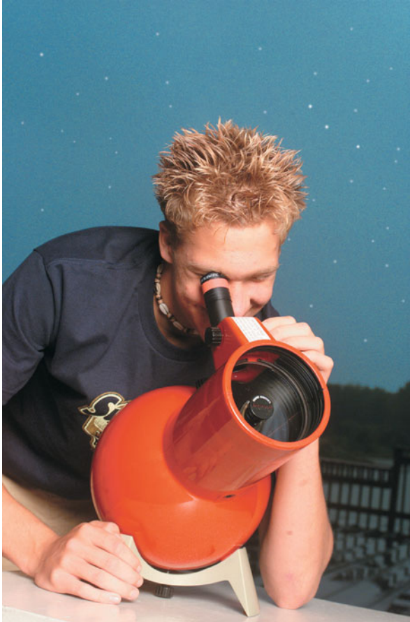
Fig. 5.5 The 4.25-in. aperture Edmund Scientifics Astroscan is one of the best-selling small reflectors ever made and it remains one of the most popular RFTs (richest-field-telescope) on the market today. It's 16 \times eyepiece provides a wide 3 ^\circ field of view (or 6 full-Moon diameters of sky), and its unique optical window protects the system from dust as well as supports its diagonal mirror. Courtesy of Edmund Scientifics
