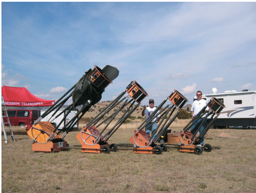
Fig. 16.1 A battery of large Dobsonian reflectors manufactured by Obsession Telescopes seen at one of the many local and national star parties that are so popular with stargazers today. Obsession’s large “Dobs” are widely considered to be the “Cadillac” of such instruments due to their excellent optics and fine workmanship. Courtesy of Obsession Telescopes
