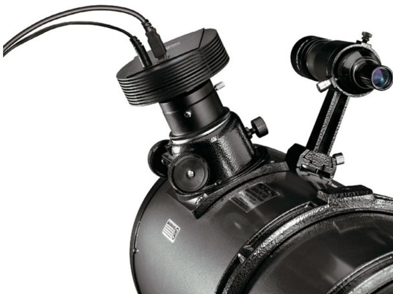
Fig. 14.3 Shown here is a CCD color imaging camera attached to the focuser of a Newtonian reflector. This one is intended primarily for use on deep-sky objects while other models are available for imaging solar system targets like the Moon and planets. In either case, the output is fed into a PC for viewing and processing. These state-of-the-art devices make it possible for amateur astronomers to routinely take pictures rivaling those of the professional observatories! Courtesy of Orion Telescopes & Binoculars
