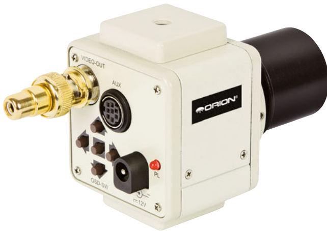
Fig. 14.1 Electronic eyepiece cameras (both black & white, and color) like that seen here make video imaging easy and affordable today. The camera output can be displayed in real time on a monitor, or recorded on a VCR or camcorder for viewing later. Courtesy of Orion Telescopes & Binoculars
