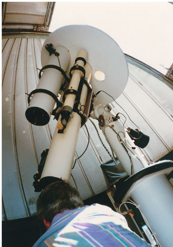
Fig. 11.3 The author at the working end of a 6-in. refractor equipped with a hydrogen-alpha solar filter. Note the circular disk at the top of the tube (through which the filtered objective end of the telescope itself protrudes) covering both the finder and an auxillary short-focus reflector (a very important precaution!). This also serves to block direct sunlight from falling on the observer. Photo by Sharon Mullaney
