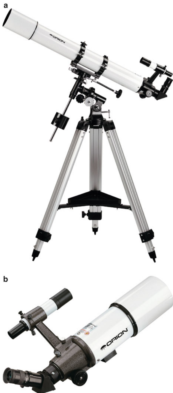
Fig. 3.1 (a, b) The long and short of it! Shown at above is a relatively long 90 mm refractor having a focal ratio of f/10 while at below is an 80 mm refractor (less than half an inch smaller in aperture) with an f/5 ratio, resulting in a much more compact instrument. Courtesy of Orion Telescopes & Binoculars
