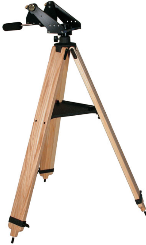
Fig. 3.3 An extremely sturdy, well-made altazimuth fork mounting with wooden tripod legs (which are preferred over metal ones for damping vibrations). Courtesy of Tele Vue Optics
