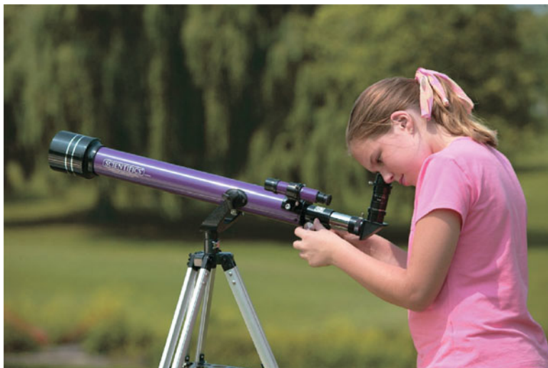
Fig. 1.1 Given good optics, even a small telescope can provide a lifetime of celestial viewing pleasure for people of all ages. Shown here is the ubiquitous 2.4-in. (60 mm) refractor, which has long been (and continues to be) the most common telescope in the world. Courtesy of Edmund Scientifics
