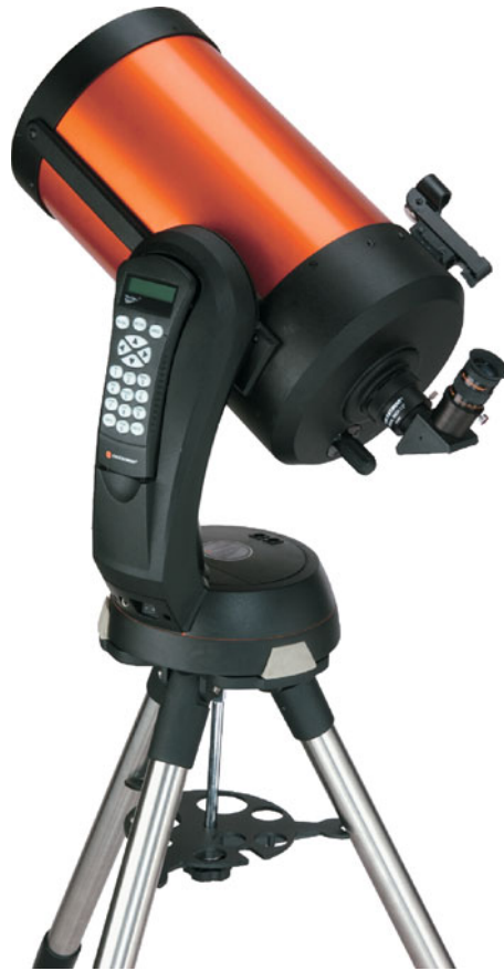
Fig. 6.5 Today's reincarnated version of the original classic orange-tubed 8-in. Celestron Schmidt-Cassegrain catadioptric that started the explosive popularity of compound telescopes. It now has such modern features as a sleek single-arm "fork" altazimuth mount and computerized Go-To acquisition of targets and tracking. Courtesy of Celestron
