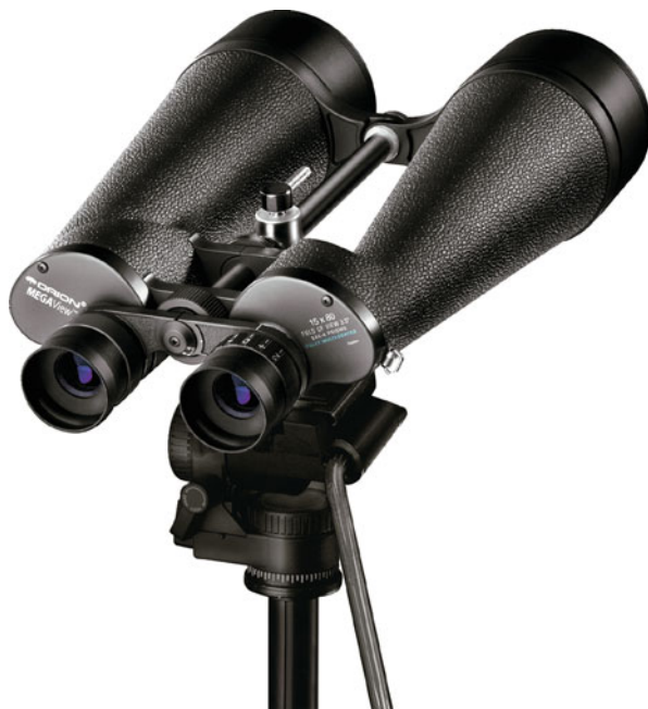
Fig. 2.3 A 15×80 giant binocular for serious two-eyed stargazing! Note, as seen here, that such large glasses must be tripod-mounted since they are much too heavy to hold steady by hand. Jupiter’s disk, the egg-shaped outline of Saturn and its rings, plus hundreds of spectacular deep-sky objects (including the brighter galaxies) lie within reach of giant binoculars. Courtesy of Orion Telescopes & Binoculars
