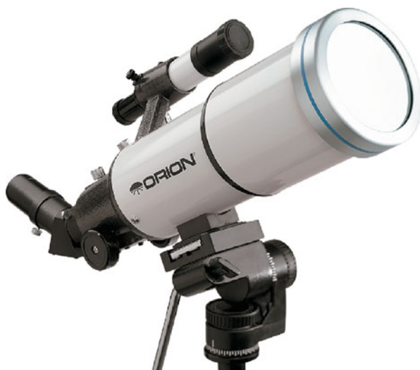
Fig. 11.1 A full-aperture optical glass solar filter mounted over the objective of an 80 mm refractor. (Note the capped finder—a very vital precaution!) While more expensive than Mylar solar filters, these provide better image contrast and a more natural looking yellowish-orange Sun rather than a blue one. Securely mounted, such full-aperture devices are completely safe for viewing our Daytime Star—in contrast to the highly dangerous practice of placing a filter over the eyepiece itself. Courtesy of Orion Telescopes & Binoculars
