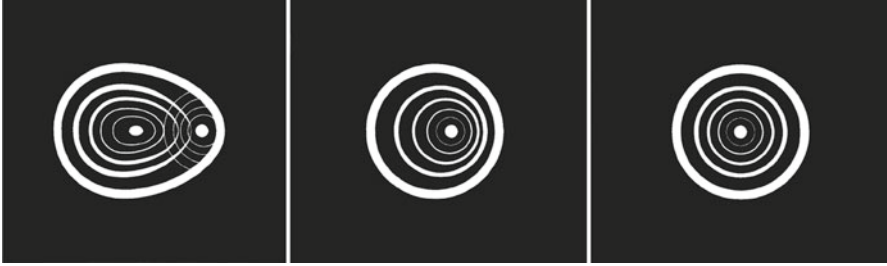
Fig. 1.3 The out-of-focus (extrafocal) image of a star can reveal many things about a telescope’s optics (as well as its thermal environment and state of the atmosphere)—in this case, the alignment of the optical components. The image in the left-hand panel reveals gross misalignment. That in the middle one shows moderate misalignment (still enough to degrade image quality), while the image in the right-hand panel indicates perfectly collimated optics
