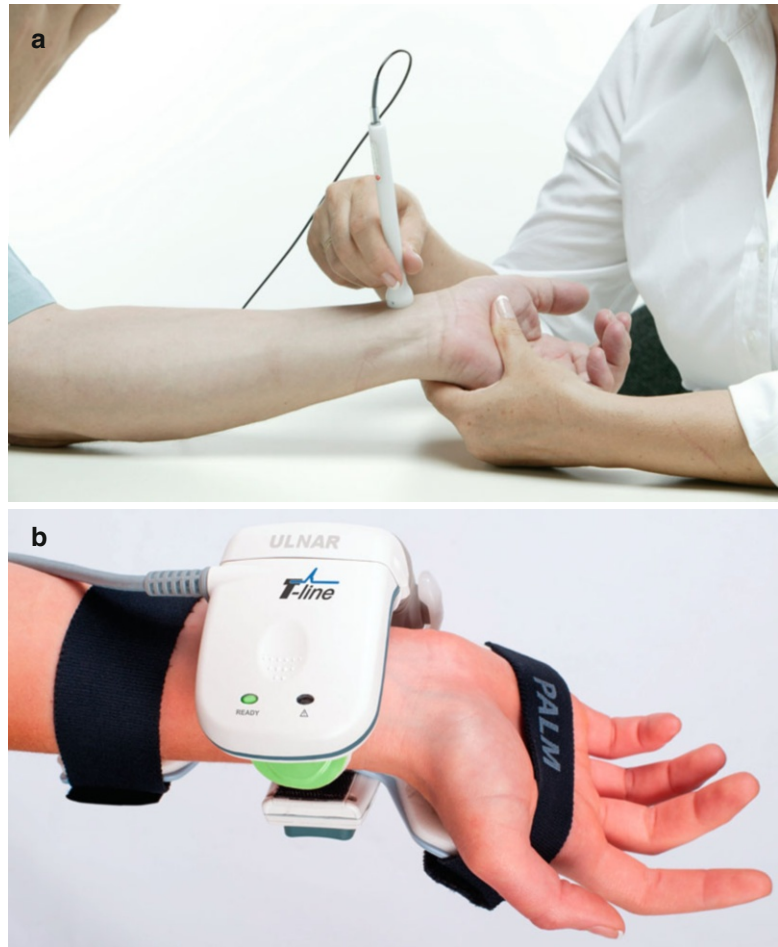
Fig. 12.5 (a) Manually operated tonometric device (SphygmoCor, AtCor Medical, Sydney, Australia) placed over the radial artery. (b) Automatic tonometric device (T-line, Tensys Medical, San Diego, USA) placed over the radial artery
