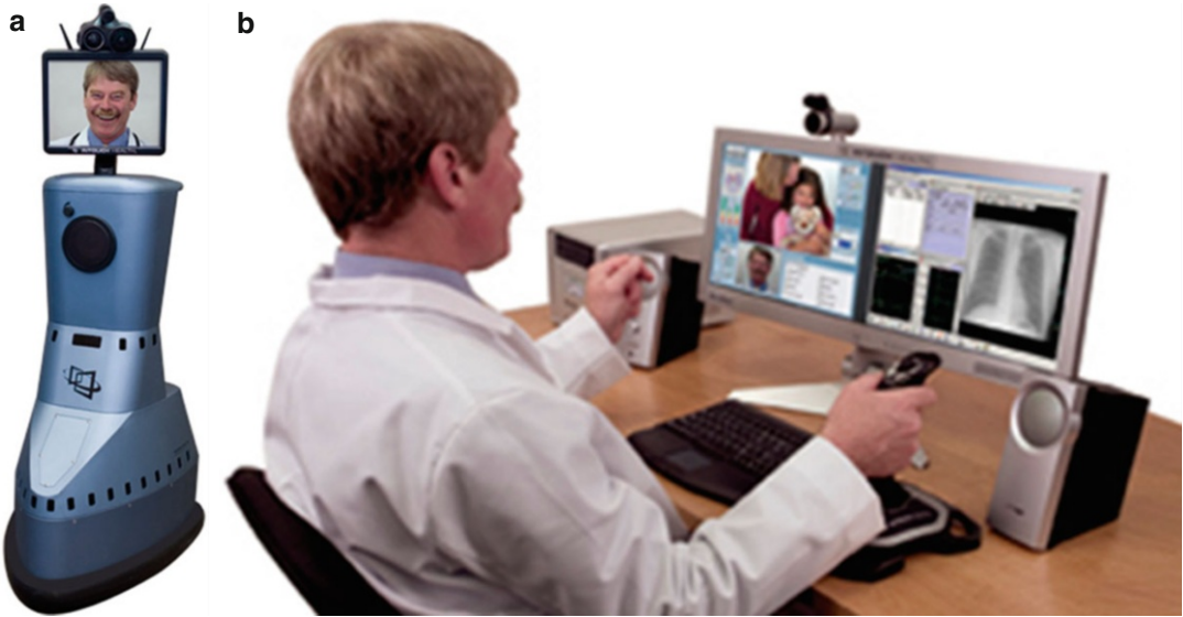
Fig. 48.1 (a) The InTouch RP-7 robot allows mobile audio-video communication with health-care professionals or patients from a remote location; communication
