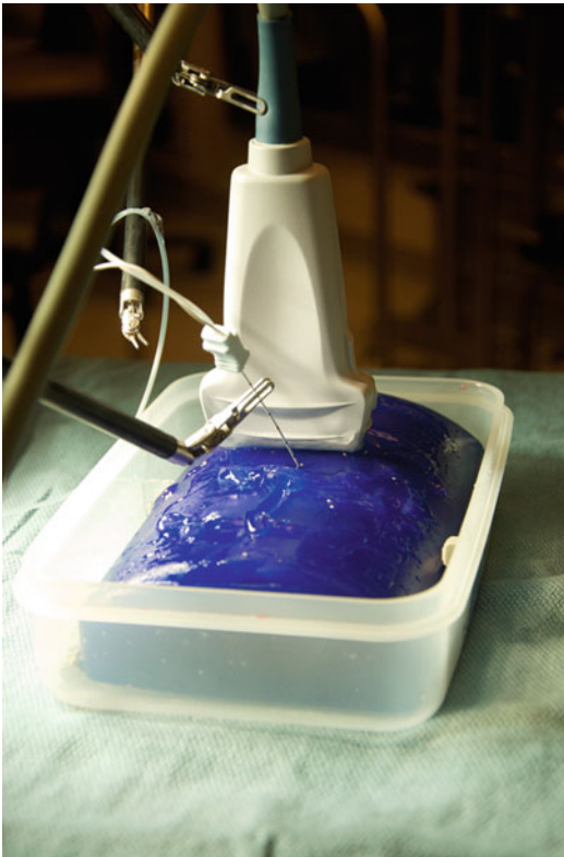
Fig. 48.7 Use of the da Vinci surgical robot for nerve blocks in a phantom
