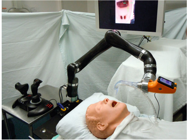
Fig. 48.6 Kepler intubation system consisting of joystick, robotic arm, and videolaryngoscope
