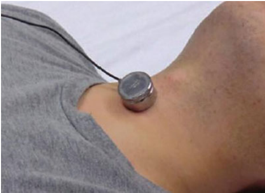
Fig. 24.8 Microphone attached to neck anterior to trachea (Reprinted with permission from Yu et al. [35])
