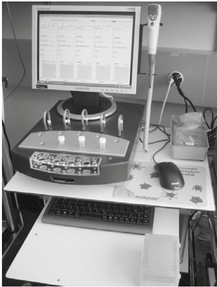
Fig. 40.2 Whole blood impedance platelet aggregometry (Multiplate). Impedance values are transformed to arbitrary aggregation units (AU), plotted against the time. In one cartridge, measurements are done in duplicates
