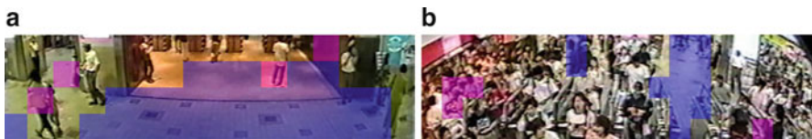
Fig. 10.5 (Color online) Observing no motion in otherwise high motion areas are also successfully detected as unusual events. Blue : true positive, Magenta : false positive, and Red : false negative
