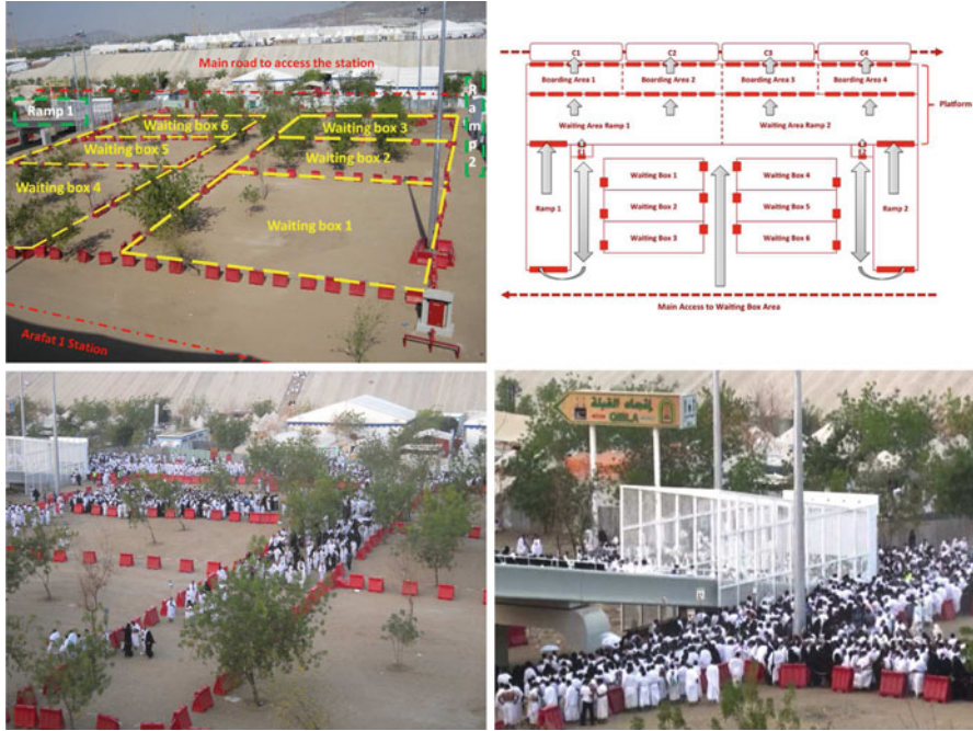
Fig. 5.4 Photos and a schematic representation of the real world scenario and the related phenomena: groups of pilgrims move from the tents area according to a precise schedule and flow into the waiting boxes, fenced queuing areas located in immediately outside the station, between the access ramps. The groups wait in these areas for an authorization by the station agents to move towards the ramps or elevators
