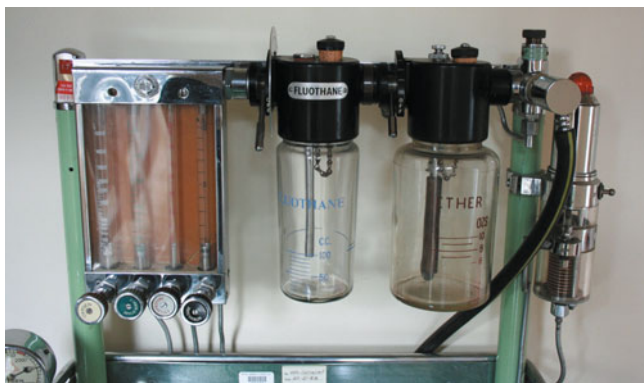
Fig. 52.7 Rotameters were used on this Boyle machine. Gas issued to the right of the flowmeter bank through valve-levers that could direct none to all of the flow through each of the two glass Boyle bottles (one here for halothane and the other for ether) in series to its right. In this photograph, the levers are down (off). Vaporization could also be increased by lowering a plunger that forced the gas directed through the vaporizing chamber to bubble through the liquid anesthetic
