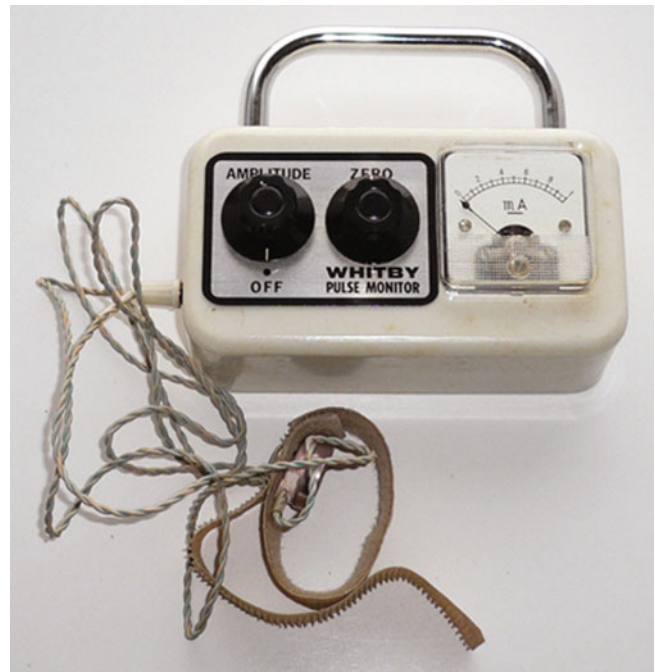
Fig. 10.4 The pulse meter, a simple device supplying a continuous visual (but not auditory) measure of pulse rate. (Courtesy of Rod N. Westhorpe.)
