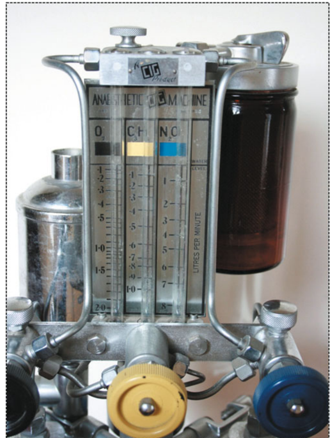
Fig. 52.3 In these CIG water depression flowmeters, the water meniscus was at the black line just above the mark indicating a 1 liter per minute flow rate when there was no gas flow. Flow depressed the meniscus non-linearly, with the greatest change occurring at the higher flows (the opposite of what might be desired)
