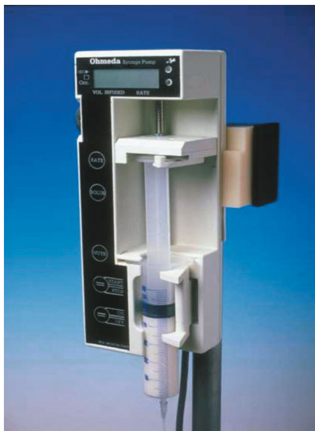
Fig. 66.5 The Ohmeda 9000 infusion pump produced by BOC Health Care in the UK in 1990 was the first of a new generation of computer controllable syringe drivers with the ability to deliver a maximum infusion rate of 200 ml/h and 'bolus' rates of 300, 600 or 1200 ml/h. (Courtesy of JB Glen)
