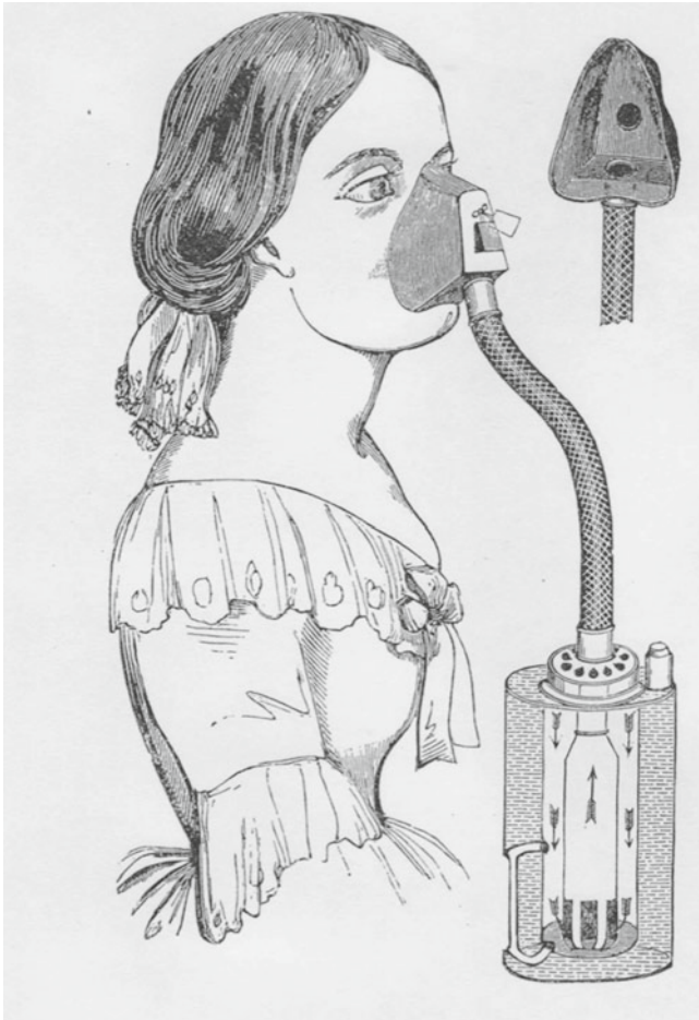
Fig. 4.3 A genteel lady breathes ether or chloroform from a vaporizer constructed to ensure the fullest concentration of anesthetic. A jacket filled with water buffers the vaporizer against temperature changes and thus against changes in the anesthetic concentration issuing from the vaporizer. A valve on the mask may be slipped more or less to one side to allow room air to dilute the anesthetic drawn from the vaporizer. When in place over the hole exiting from the mask, the valve allows no room air in but allows easy exit of the gases inspired by the patient (p 82) [12]. (From Snow J: On the Inhalation of the Vapour of Ether in Surgical Operations: Containing a Description of the Various Stages of Etherization, and a Statement of the Result of Nearly Eighty Operations in Which Ether Has Been Employed In St. George's and University College Hospitals . London: John Churchill, 1847. pp 1–88.)
