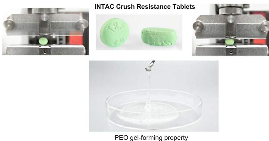
Fig. 6.2 Illustration of INTAC ® technology's resistance to tablet crushing and high viscosity gels due to POLYOX properties (Used with Permission, Grünenthal GmbH, copyright 2013)
