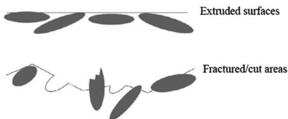
Fig. 13.25 Schematic representation of extruded surfaces and fractured/cut areas. (Reproduced from Reitz et al. 2008, with permission from Elsevier)
