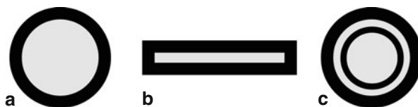
Fig. 12.6 Schematic representation of various extrusion die shapes
