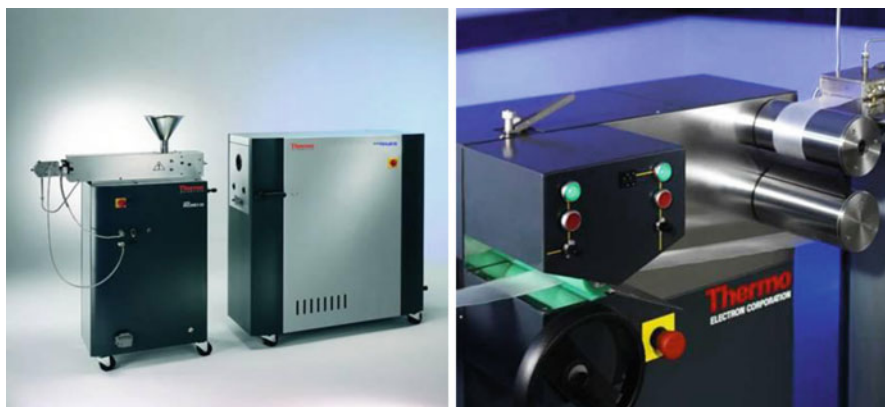
Fig. 12.2 Single-screw extrusion— left : Thermo Fisher Scientific PolyLab OS Torque Rheometer System coupled with a single-screw extruder and film die for sheet profile manufacture; right : A close-up of film profile extrusion with a Post-Extrusion Film Haul-Off System (reproduced with permission from Thermo Fisher Scientific)
