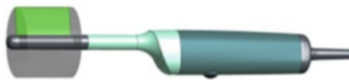
Fig. 2.13 The 8838 probe elements move within the shaft radially to create a 3D data volume
