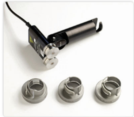
Fig. 2.10 The external mover elements for 8848 probe
