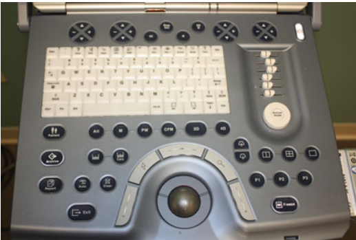
Fig. 3.14 The dominant hand generally operated the console. Unlike BK console, the GE Voluson e buttons on the console are multifunctional, and their function corresponds to the menu at the bottom of the screen © SHOBEIRI 2013
