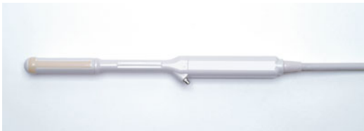
Fig. 11.15 Hitachi Aloka linear/convex endocavitary EUP-U533 probe. Frequency band: 5.0–10.0 MHz linear, 5.0–9.0 MHz radial. Linear length/radius/sector angle: 64 mm/10 mm/200°. Depth of field of view: 30–170 mm. Display modes: B-Mode, M-Mode, PW, CFM, CFA, dTHI, WPI
