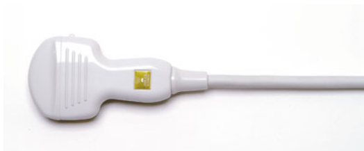
Fig. 11.12 Hitachi Aloka 3D abdominal convex probe EUP-C524 used for transperineal imaging. Frequency band: 3.5–7.5 MHz. Radius/angle: 40 mm/70°. Depth of field of view: 40–210 mm. Display modes: B-Mode, M-Mode, PW, CFM, CFA, dTHI, WPI
