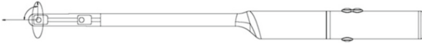
Fig. 2.8 The 2052 probe has two buttons on the handle anteriorly that allows manual pilot of the scanner elements within the probe. The button posteriorly activates the probe or freezes the image on the screen
