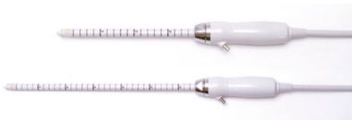
Fig. 11.9 Hitachi Aloka R54 probe: Frequency band: 5.0–10.0 MHz. Radius/sector angle: 6 mm/270°. Depth of field of view: 30–170 mm. Display modes: B-Mode, M-Mode, PW, CFM, CFA. Probe length: 190 and 330 mm, adaptable with rectoscope
