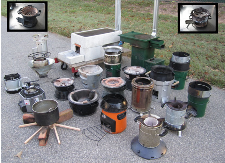
Fig. 13.2 Display of multiple cookstove types used around the world. This photograph shows the wide variety of cookstoves using solid fuels in LMIC including: Open “3-stone” fire, wood fuel, Berkeley Darfur, wood fuel, Envirofit G-3300, wood fuel, Onil, wood fuel, Philips HD4008, wood fuel, Philips HD4012, wood fuel, Sampada, wood fuel, StoveTec GreenFire, wood fuel, Upesi Portable, wood fuel, GERES, charcoal fuel, Gyapa, charcoal fuel, Jiko, ceramic, charcoal fuel, Jiko, metal, charcoal fuel, KCJ Standard, charcoal fuel, Kenya Uhai, charcoal fuel, StoveTec prototype, charcoal fuel, Belonio Rice Husk Gasifier, rice hull fuel, Mayon Turbo, rice hull fuel, Oorja, biomass pellet fuel, StoveTec TLUD prototype, wood pellet fuel, Jinqilin CKQ-80I, corn cob fuel, and Protos, plant oil fuel (Courtesy of James Jetter, U.S. EPA, National Risk Management Research Laboratory Air Pollution Prevention and Control Division, Stove Testing Center, Research Triangle Park, North Carolina, USA)
