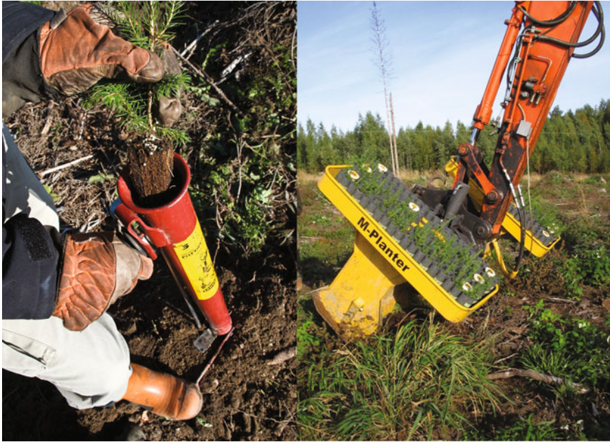
Fig. 2.9 Planting can be done by hand with a planting tube or by machine. (Photo: Erik Viklund and Karin Johansson)
