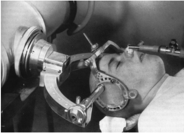
Fig. 1.2 First stereotactic instrument for radiosurgery using 280 kV X-rays, early 1950s. From Textbook of Stereotactic and Functional Neurosurgery . Lozano, Andres M.; Gildenberg, Philip L.; Tasker, Ronald R. (Eds.) 2nd ed. 2009; used with permission
