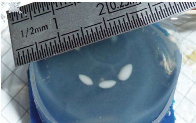
Fig. 11.3 Heated zones produced after insonification in thermosensitive gel around the focal zones after several seconds of exposure
