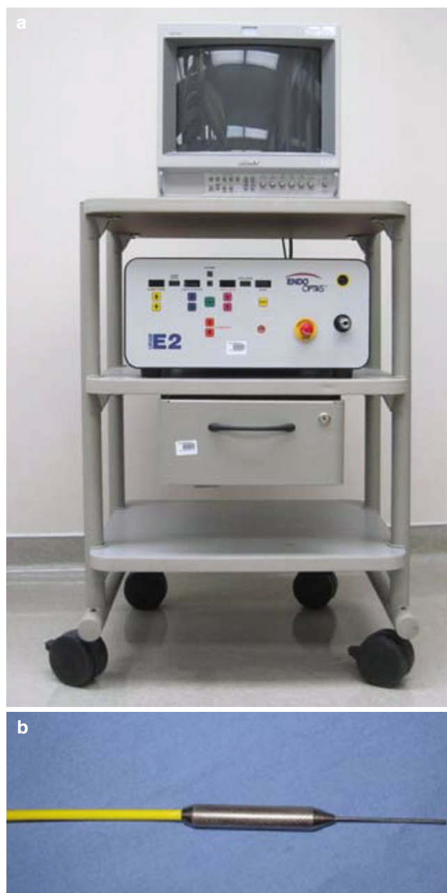
Fig. 9.2 (a) ECP unit (Uram E2, Endo Optiks, Little Silver, NJ), including laser and monitor. (b) ECP probe (20 gauge)
