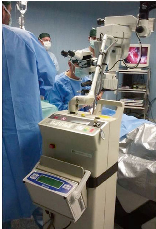
Fig. 10.1 CLASS OT-135 system ("IOptiMate"; IOptima Ltd., Ramat Gan, Israel) consists of a Beam Manipulator System conjugated with a CO 2 laser
