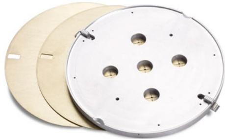
correction. The phantom has an outer diameter of 22.78 cm and thickness of 1.28 cm. It weighs 1.86 kg (Fig. 6.19).
