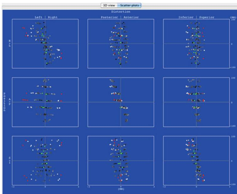
**Fig. 10.10** An image distortion plot generated using Image Owl (Salem, NY) MR Distortion Service. The Magphan<sup>®</sup> Quantitative Imaging Phantom is scanned, and the DICOM image set is uploaded for processing. Actual and imaged sphere positions are evaluated to provide fourth-order distortion measurements
