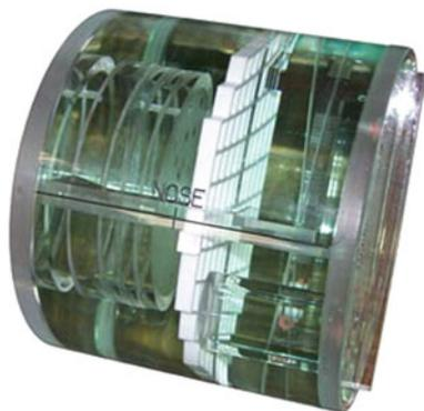
**Fig. 10.3** ACR small knee phantom, 100 mm (length)  $\times$  100 mm (diameter)
