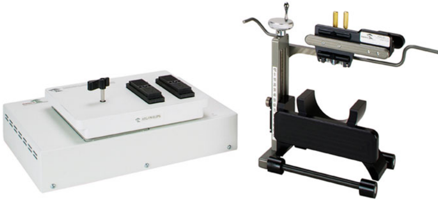
Fig. 9.8 Example of an electronic ultrasound test device—the ultrasound transducer is mounted on the stand to the right and placed in a water tank. The probe is connected to the box on the left which is controlled by a computer. Individual “pings” of elements of the transducer produce echoes which bounce back from the reflector (this is configured for a curvilinear probe) and processed to determine which elements are operational
