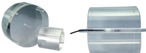
Fig. 7.1 Head and body CT dosimetric phantom manufactured by Radcal Corporation. The phantoms are composed of cylindrical massive blocs of PMMA containing holes dimensioned for the exact introduction of pencil ion chambers
