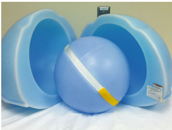
Fig. 10.12 A photograph of the magnetic field homogeneity phantom issued by General Electric Healthcare (Waukesha, WI) during installation of the MRI system
