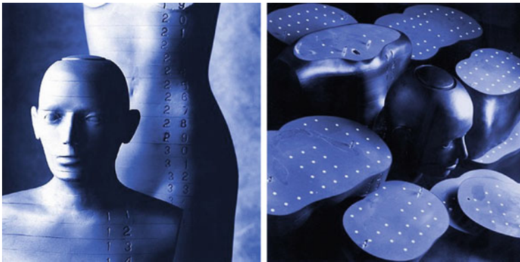
Fig. 7.8 The RANDO ® phantom manufactured by The Phantom Laboratory. The phantom is composed of a proprietary urethane formulation for mimicking human soft tissue [55]
