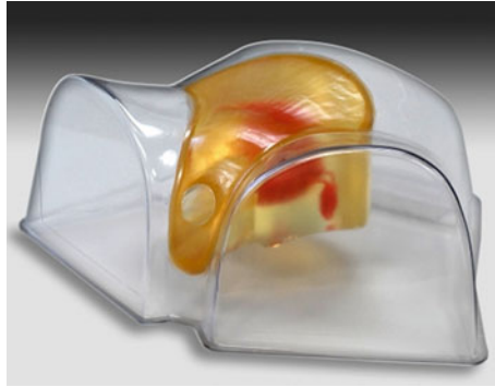
Fig. 5.3 The model 404 female pelvis ultrasound training phantom by CIRS, Inc. http://www.cirsinc.com/products/new/91/female-ultrasound-training-pelvis/ . This phantom could potentially be modified to serve as a training phantom for gynecological brachytherapy, inserting cylindrical applicators, tandem and ovoid applicators, or interstitial needles
