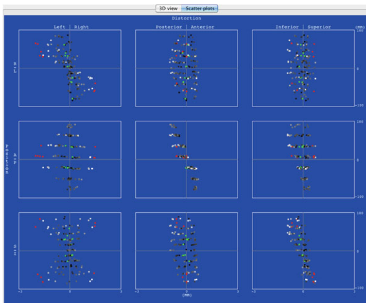
Fig. 10.10 An image distortion plot generated using Image Owl (Salem, NY) MR Distortion Service. The Magphan ® Quantitative Imaging Phantom is scanned, and the DICOM image set is uploaded for processing. Actual and imaged sphere positions are evaluated to provide fourth-order distortion measurements
