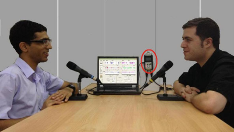
Fig. 34.2 Recording system consisting of the Zoom H4n voice recorder ( circled in red ) and two Sennheiser e845s microphones, one for each participant in the conversation. The laptop can run the GUI (cf. Sect. 34.3.3), which can be used to provide real-time non-verbal speech statistics to an external observer
