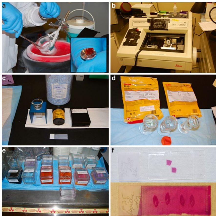
Fig. 6.2 (a) Snap-freezing of fresh tissue sample on a cryostat sample holder. (b) A Leica CM3050 Cryostat for cryosectioning of sample and collection onto slides pre-coated with emulsion. (c) Dip Miser slide coating cup (Electron Microscopy Sciences, Inc.), Kodak emulsion, black slide exposure box, Drierite desiccant and a coated slide. Slides are dipped into liquid emulsion heated in the Dip Miser and allowed to dry. Sections are collected onto the pre-coated slides and tissue sections are exposed in a sealed black slide box with desiccant at 4 °C. (d) Slides are developed using Kodak Developer and Fixer. (e) Slides may be stained as usual. (f) Examples of slides that have been stained; note the bottom slide shows how emulsion picks up stain, while the upper slide has no emulsion coating (from Solon, in Braddock 2012)
