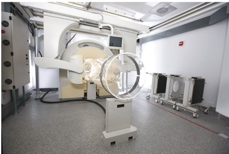
Fig. 10.3 Photograph of the SPECT/CT equipment with containment extension tube
