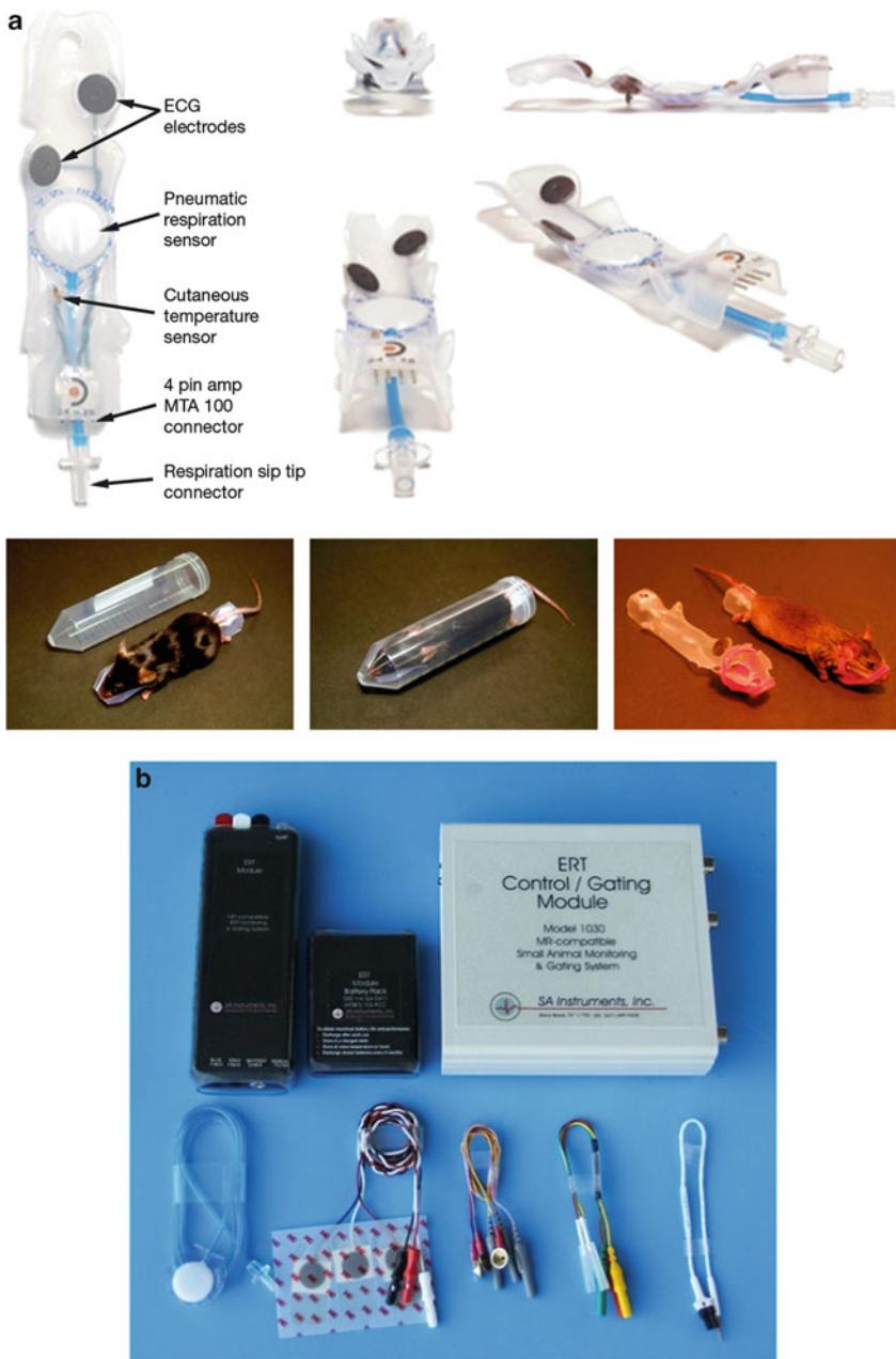
Fig. 7.1 (a) DAZAI system where specific beds are molded to mice of differing body weights and the resulting “sled” is fitted with ECG, respiration, and thermocouple sensors for full physiological monitoring of an animal’s well-being while under anesthesia. (b) SAII system integrated with the DAZAI system, the SAII monitoring hardware allows the physiological signals to be electronically traced and stored; furthermore, integrating this system into the MRI or PET hardware enables the operator to gate/trigger acquisitions to cardiac and/or respiration cycles
