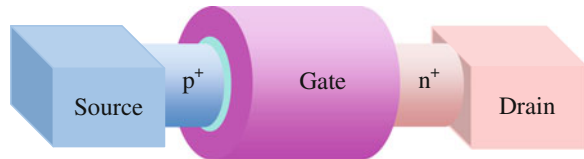
Fig. 7.17 Schematic diagram of a horizontal nanowire TFET structure
