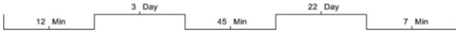
Fig. 25.3 Symbols depicting process and wait time duration in VSM. These typically appear on the bottom third of the VSM. Symbols created in eVSM (eVSM.com)
