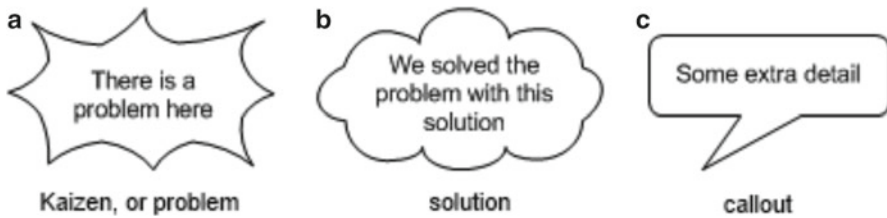
Fig. 25.4 Additional descriptive symbols used in VSM. These can appear anywhere on the diagram, as needed. Symbols created in eVSM (eVSM.com)
