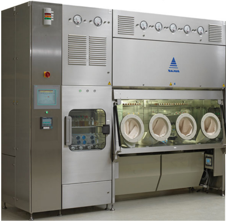
Fig. 9.3 VHP airlock located next to an isolator (courtesy from Skan AG)
