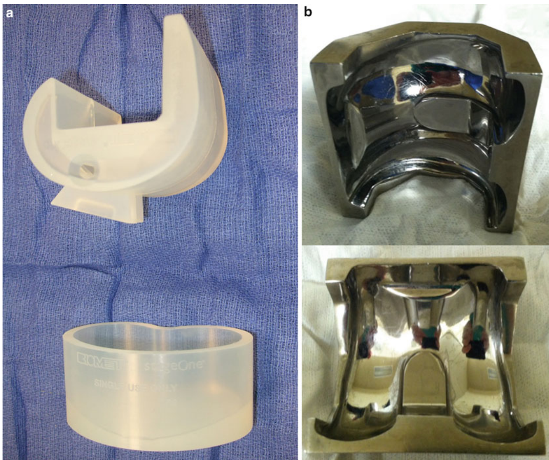
Fig. 16.2 (a) Photograph of commercially available spacer molds. (b) Photographs of custom made cast stainless steel spacer mold
