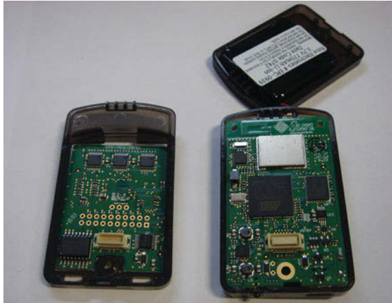
Fig. 24.2 The different layers of a Sun SPOT
