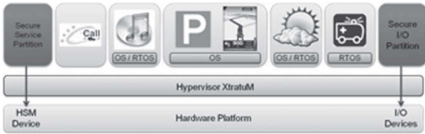
Fig. 12.3 OVERSEE vehicular security architecture
