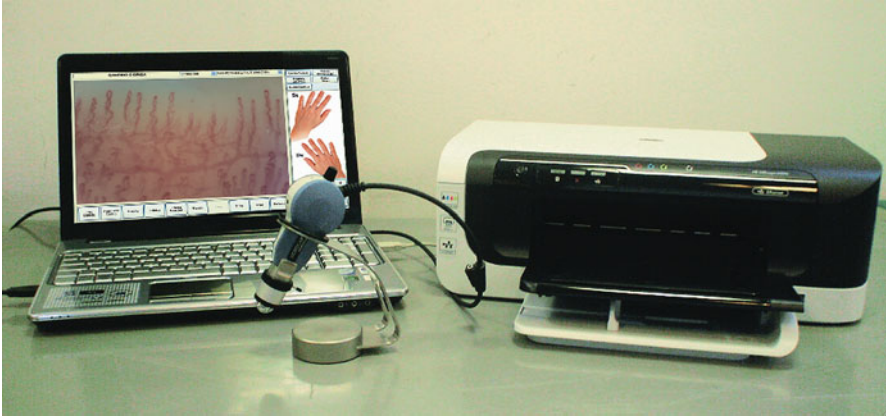
Fig. 11.1 A videocapillaroscope that is used in detecting the microcirculation at the level of the nailfold bed
