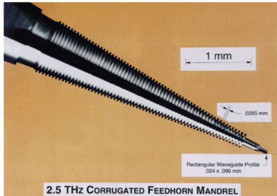
Figure 31.2: Example of state-of-the-art micro-machining: a mandrel for a corrugated feedhorn at 2.5 THz with structures as small as 26 \mu\text{m} . (Courtesy B. Ellison, RAL).
