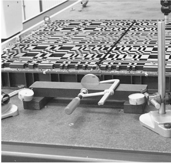
Figure 12.2: Uniformly redundant array mask on INTEGRAL /IBIS (adapted from http://integral.esac.esa.int ).
