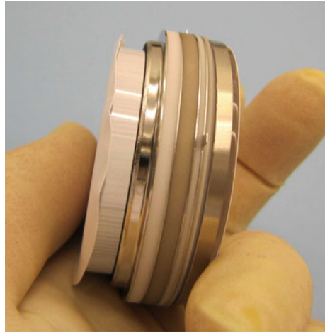
Figure 25.2: An image intensifier tube with input window and output fibre block (made by ProxiVision GmbH, Germany).
