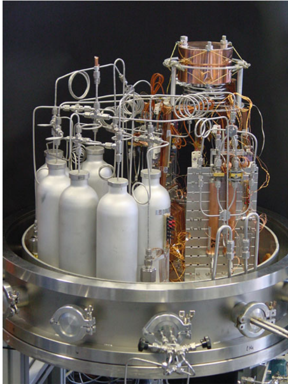
Figure 37.5: 4 K sorption-cooler prototype under development (Univ. Twente).
