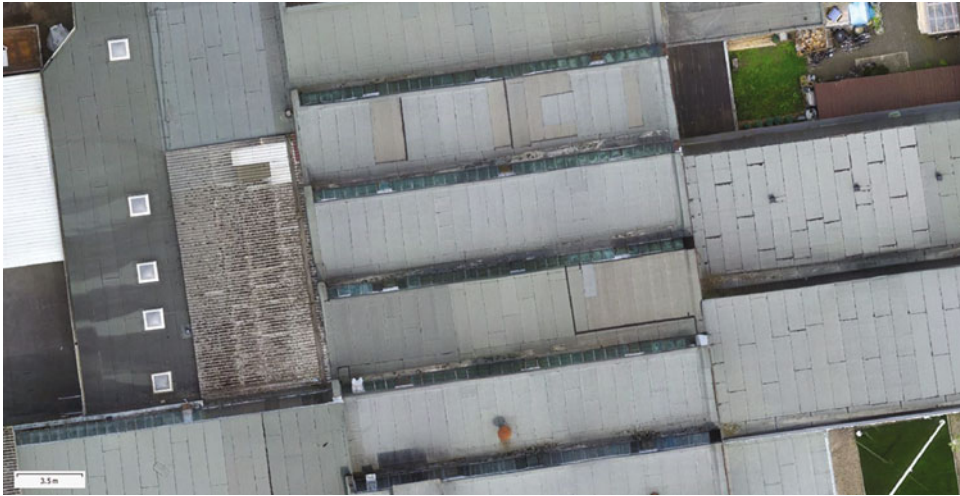
Geodesy, Fig. 13 Roof landscape as an orthophoto (acc. <\pm 1 mm) captured by UAV
