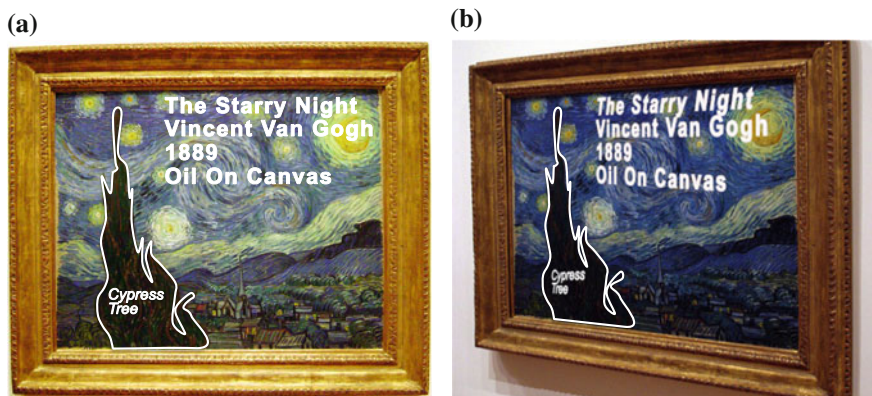
Fig. 5.3 Example of AR. a Reference frame with the additional information to display. b Current frame with the additional information transformed using the feature-based homography transformation
