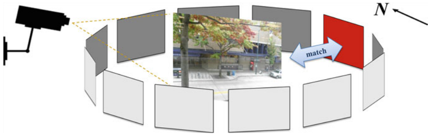
Fig. 9.3 The estimation of principal orientation of the camera
