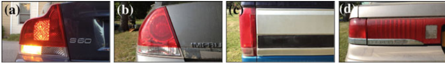
Fig. 6.15 Examples of domestic non-segmented and foreign segmented taillights. a Volvo turn. b Chevrolet Impala. c Ford F-150. d Mercury Cougar
