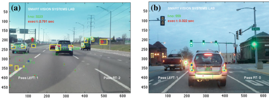
Fig. 6.3 Dawn and Dusk scenarios. Note the high number of false-positives (due to relaxed color thresholds), which are later successfully eliminated by the algorithm. a Dawn scenario. b Dusk scenario
