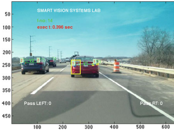
Fig. 6.7 Elimination of a red vehicle chassis using symmetry. The red chassis is asymmetrical to other objects in the frame
