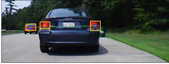
Fig. 6.8 Incorrect detection of “symmetrical” light pairs without the use of 3-dimensional histograms ( red passing car and right taillight)
