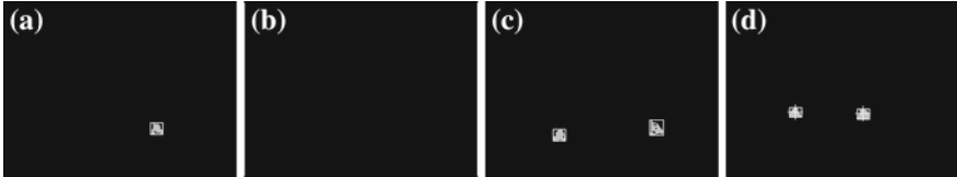
Fig. 6.17 Different detection scenarios. a Missing 1 light, b missing both, c tracker not upd. d Tracker updated
