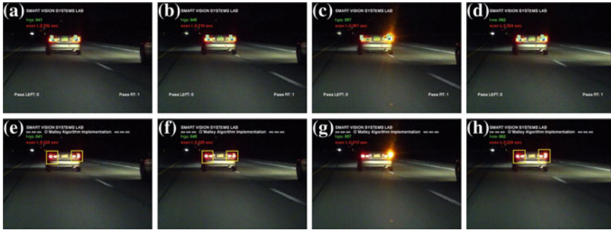
Fig. 6.20 An illustration of tracking through a turn signal using the proposed algorithm ( top row ) and the method in [22] ( bottom row ) using auto-exposure settings. The algorithm in [22] has problems when there are drastic light shape, color, and intensity changes. In addition, daytime–nighttime detection requires auto-exposure to adjust for changes in lighting conditions, whereas the approach in [22] implements the algorithm using a set exposure. a Frame 841. b Frame 845. c Frame 857. d Frame 862. e O’Malley (841). f O’Malley (845). g O’Malley (857). h O’Malley (862)
