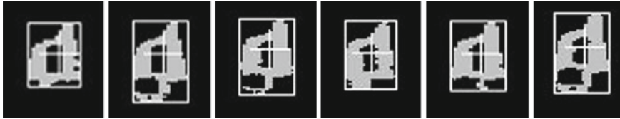
Fig. 6.16 Area change through one complete cycle of a turn signal
