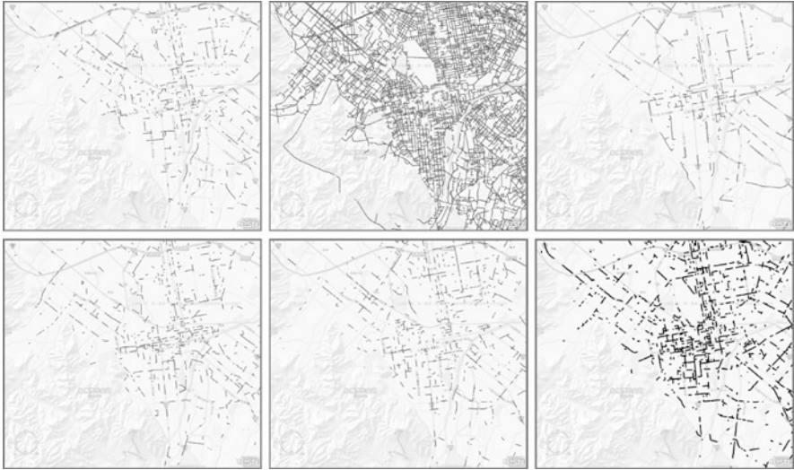
Fig. 5 Clustering result for rush hour of a day directly after a heavy snowfall. The segments from the major roads end up in several different clusters
