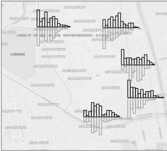
Fig. 9 Histograms showing the speed in intersections around our university. The gray bars are the speed in winter and the black bars are the speed in summer. The bar farthest to the left is 0–5 km/h, the next 5–10 km/h, etc
