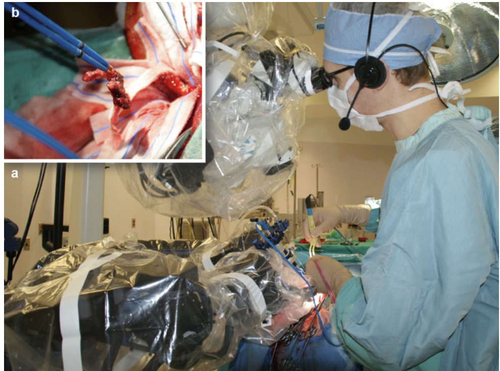
Fig. 46.5 (a) For microsurgical procedures, neuroArm is positioned at the operating table in the position of the primary surgeon. The assistant surgeon is able to operate in an ergonomic position relative to neuroArm and the operating microscope. (b) The neuroArm bipolar forceps can be used to coagulate as well as remove pathological tissue
