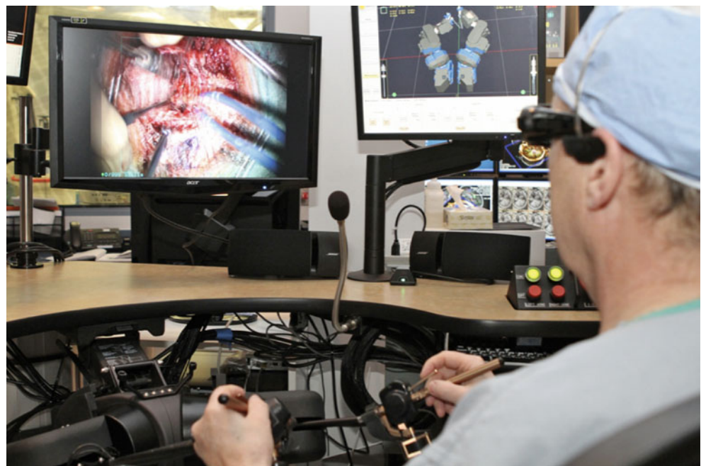
Fig. 46.4 The neuroArm human-machine interface recreates the sight, sound, and touch of the surgical site for the surgeon. The surgeon is provided with a 3-D stereoscopic view of the surgical corridor. The command status display (right of the stereoscopic display) shows the position of the neuroArm manipulators in relation to the radio frequency coil. The surgeon controls neuroArm using two modified PHANTOM hand controllers, providing seven DOF control with three DOF force feedback. The surgeon communicates with the surgical team using a wireless headset
