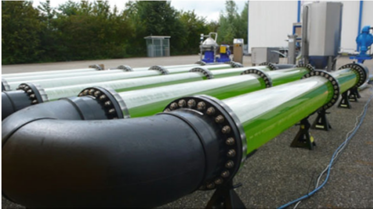
Fig. 30.13 Actual view of the tubular PBR in outdoor environment
