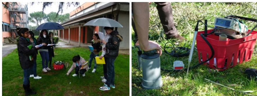
Fig. 20.3 Pupils measure the carbon dioxide emission from the soil of their school garden
