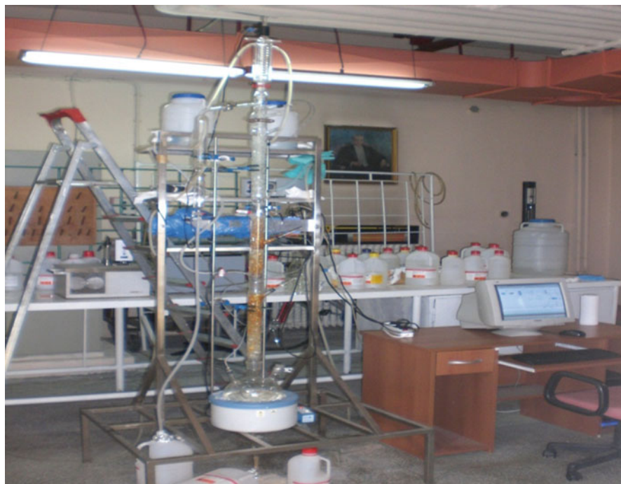
Fig. 39.7 Pictorial view of reactive packed distillation column setup
