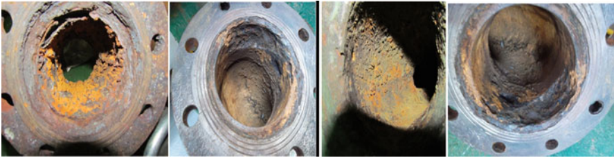
Fig. 51.10 Cavitation in fittings and in 90 and 180° elbows. (The elbow photographs viewed were taken in March 2012 at ÇanDemir Shipyard)
