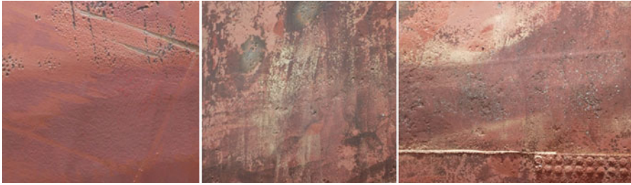
Fig. 51.11 Cavitation on vertical side of ship. (The vertical side photographs viewed were taken in May 2012 from M/V Sismik-1)
