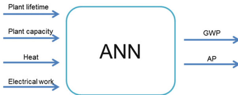
Fig. 26.12 ANN model for nuclear-based hydrogen production
