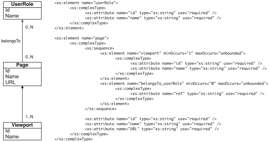
Fig. 3.6 Example of translation of a meta-model fragment into XSD
