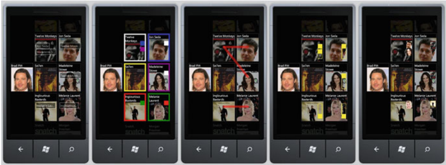
Fig. 10 Different explicit link representations. (a) Text: nodes with the same name are linked. (b) Color: nodes with the same nodes with the same color are linked. (c) Connectedness: nodes with lines between them are linked. (d) Proximity: nodes at/containing the same vertical position are linked. (e) Texture: nodes with/containing the same image are linked
