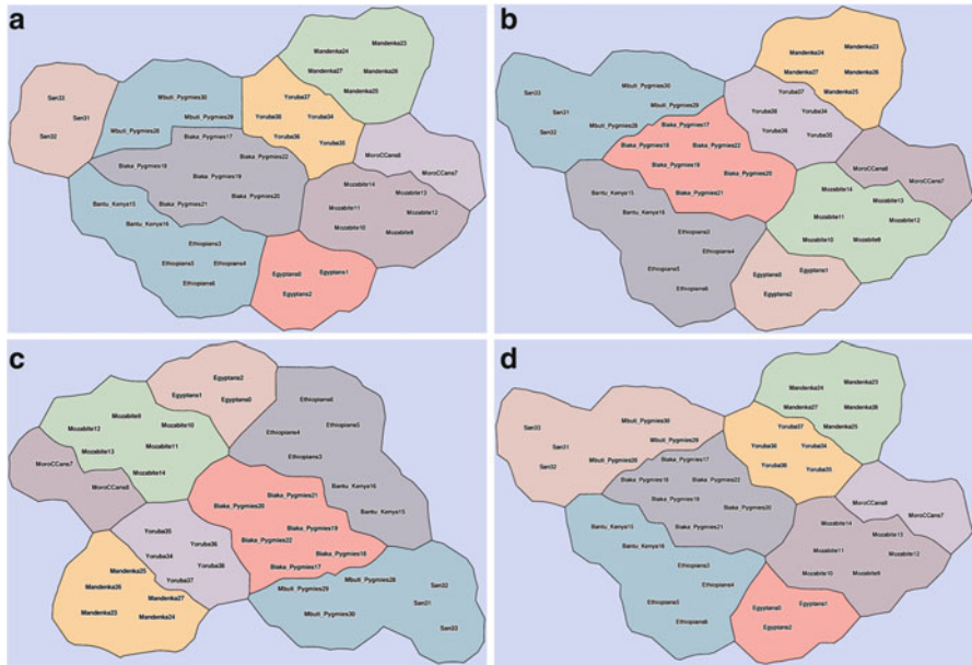
Fig. 9 Visualizing multiple maps requires both layout stability and color stability. (a): original map. (b): a new map based on different similarity data, and with node layout computed independently. It is difficult to see the corresponding nodes in the two maps. (c): the new map computed to optimize node layout stability with regard to (a), which makes it possible to compare nodes, while clusters are still hard to compare. (d): the new map with optimal node layout and color assignments, which makes it easy to compare with (a); e.g., it is clear that two clusters in the top left of (a) are now merged
