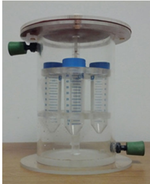
Fig. 28.9 Custom-designed holder for MR imaging of tissue specimens
