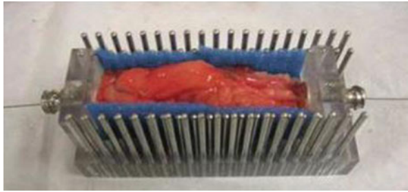
Fig. 26.57 Tissue cage fixture: the artery is fixed in the cage and an automatic pullback is performed in saline and human blood. The histology sections are taken at every 2 mm using side rods after the artery was fixed by formaldehyde [32]
