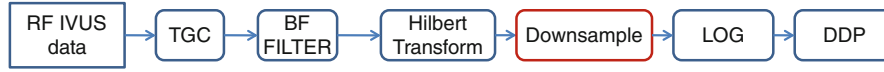
Fig. 13.4 Image reconstruction process. A Time Gain Compensation (TGC) operation is applied to the RF IVUS data acquired. The envelope is recovered by a Hilbert Transform. A downsample stage is applied to obtain isotropic resolution, all the analysis of this work is applied after
