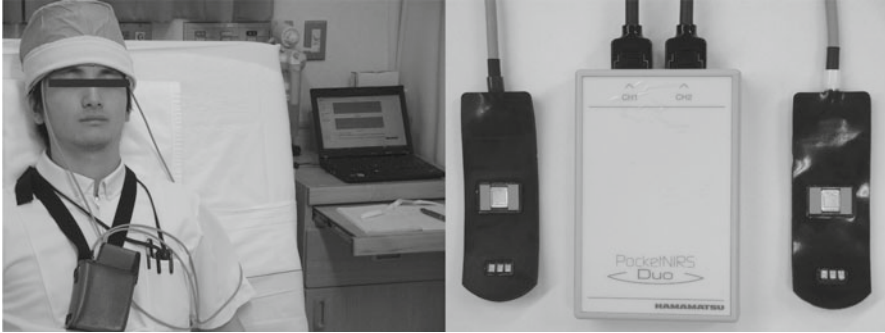
Fig. 62.1 The NIRS system uses LEDs of three different wavelengths (735, 810, and 850 nm) as light sources and one photodiode as a detector; it has two channels. The total weight of the controller and probes is only 160 g. The sampling rate was 61.3 Hz (i.e., the sampling time was about 16.3 ms)
