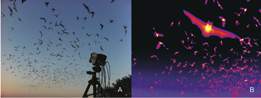
Fig. 8.5 Thermal imaging can be used to produce high-contrast, high-resolution imagery that can be used by a variety of researchers. (a) A visual light image of Tadarida brasiliensis emerging from Frio Cave. Thermal cameras are arranged such that their field of view includes the bats with a backdrop of the sky. (b) The resulting images provide unprecedented detail of bat flight and group behavior (photo credit N.W. Fuller)
