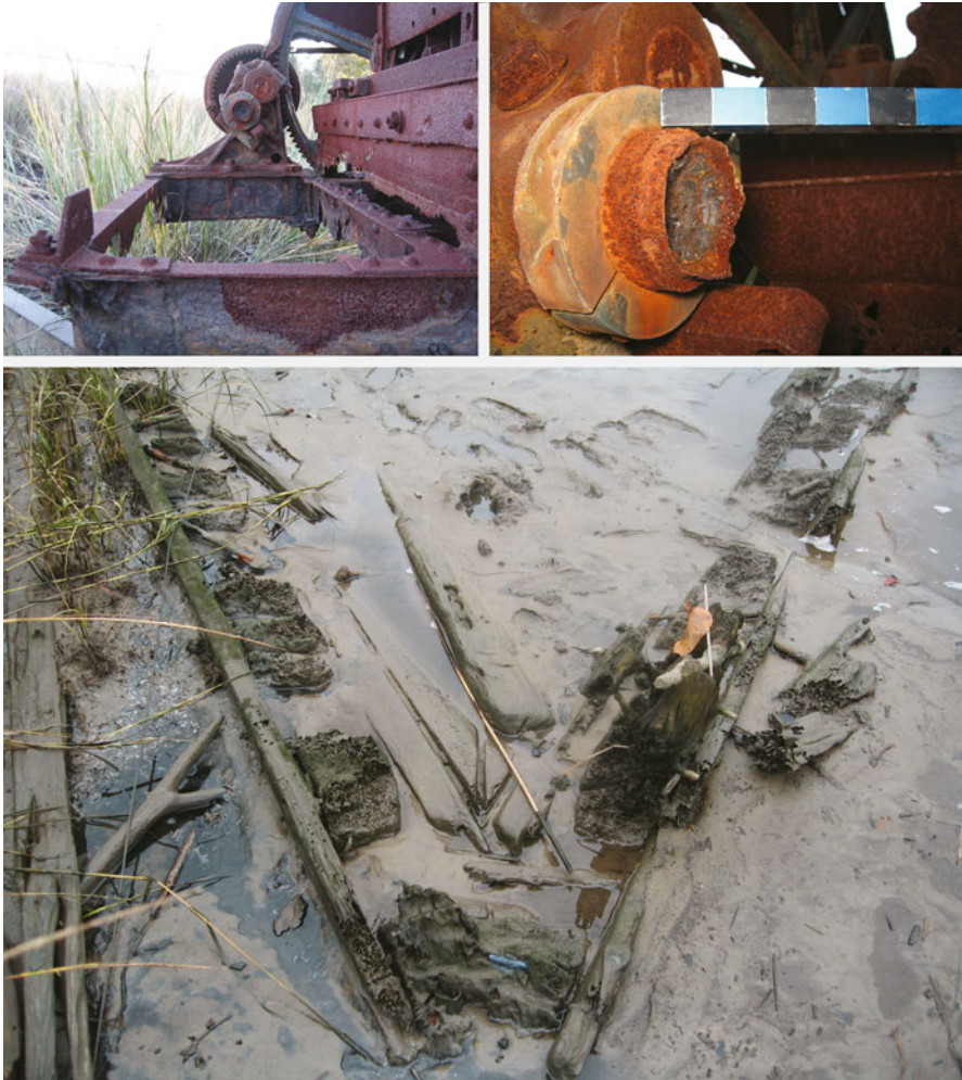
Fig. 12.4 Signatures of salvage appear through evidence of cutting. On Steam Crane Barge 3, an empty engine mount ( top left ) and evidence of cutting on the crankshaft ( top right ). (Images by Sami K. Seeb). Bottom On Waccamaw , cut marks can be seen on the wood in the bow. (Image by Nathan Richards)
