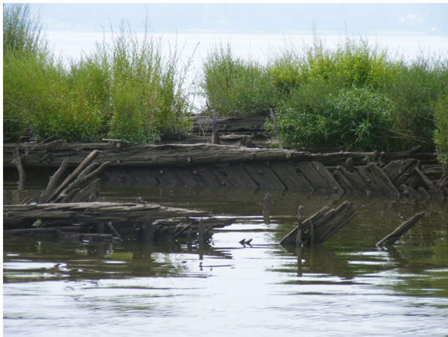
Fig. 5.2 Construction details of a combination barge with diagonal ceiling planking. (Courtesy Joshua A. Daniel)
