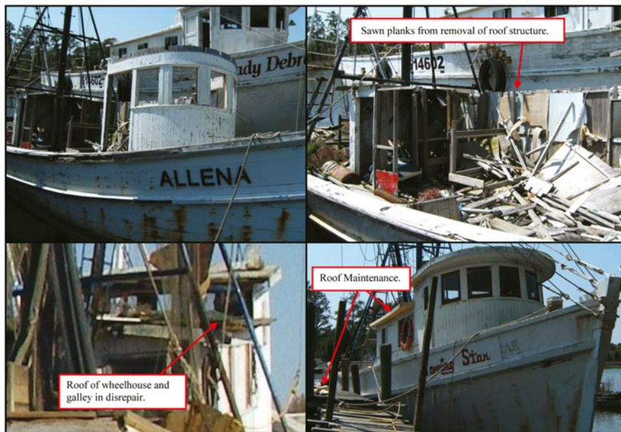
Fig. 11.5 Vessel 24 ( Miss Allena ) top-left and top-right undergoing salvage for recycling. Working vessel Morning Star ( bottom left and bottom right ), utilizing Vessel 24's recycled material with new lumber to facilitate maintenance of wheelhouse and galley. (Photo by Jacqueline Marcotte, 2010)
