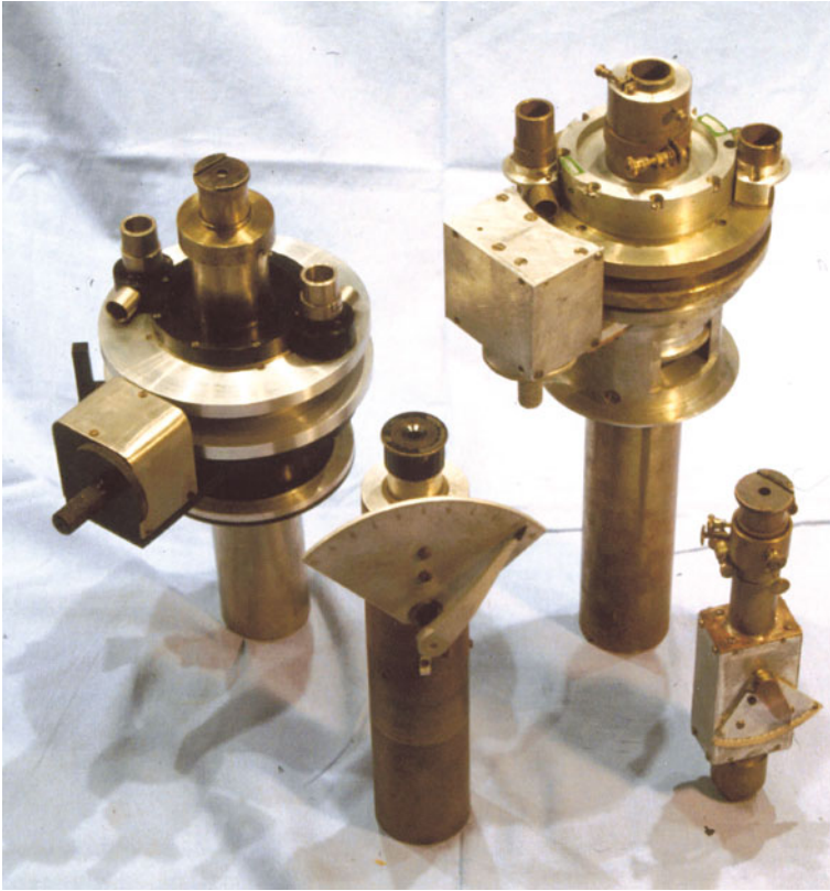
Fig. 9.11 Double image micrometers for the measurement of planetary bodies. Front centre: B. Lyot's apparatus for close double imaging, designed in 1941. Rear right: micrometer for wide double imaging of A. Dollfus, the prototype from 1952, and its accessory for photometry of planetary surfaces. Rear left: the Dollfus micrometer in its commercial version made by the firm of R. Danger
