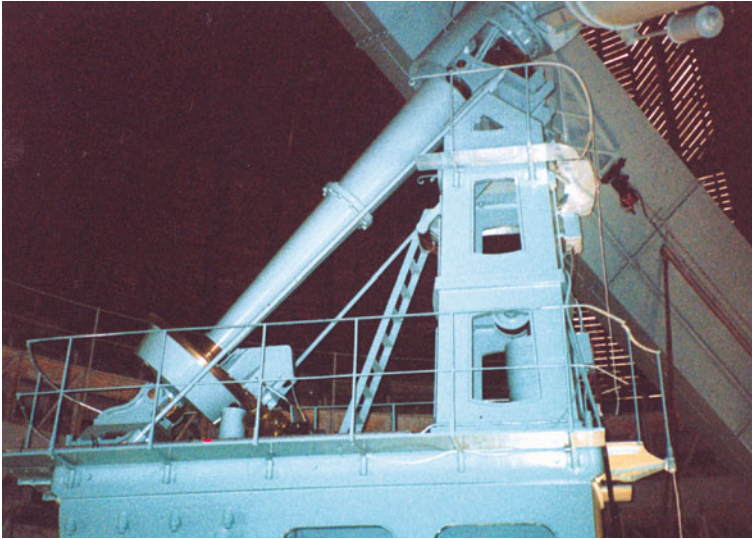
Fig. 2.5 The equatorial mounting, with the pylon carrying the upper landing, the footbridge surrounding the mounting and the upper footbridge above around the landing
