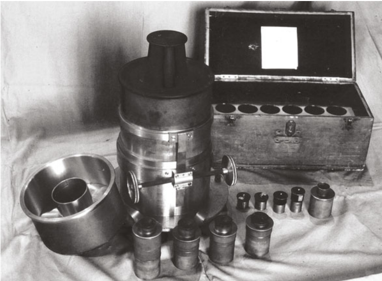
Fig. 3.2 The eyepiece box for the Grande Lunette, the set of eyepieces (the four smallest ones are not originals) and the large rack mount holding the eyepiece giving a wide, bright field
