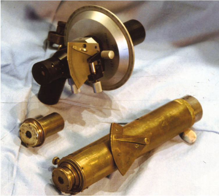
Fig. 7.1 Lyot's visual fringe polarimeter. In the foreground, the prototype of Lyot's apparatus together with its polariscopic eyepiece, used with the Grande Lunette by its creator from 1924 to 1928. In the background, the version of the instrument made by the société Jobin and Yvon, used with the Grande Lunette by J. Focas and A. Dollfus from 1965 to 1969, then by S. Ebisawa from 1973 to 1980
