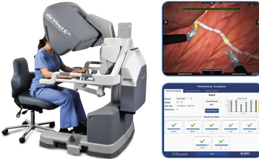
Fig. 8.2 Integrated digital simulation for computer-assisted surgical system. Clockwise from left to right : original surgical console with computer “backpack”
