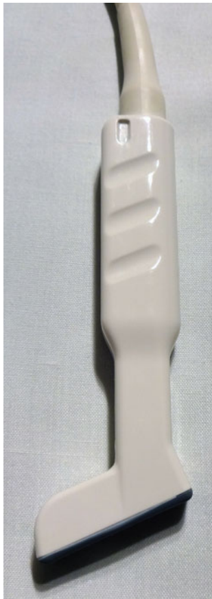
Fig. 1.2 HVFUS linear array “hockey stick” transducer. Versatile multi-frequency (up to 15 Mhz) compact ‘hockey stick’-shape transducer, with a high Doppler and color flow sensitivity. The hockey stick-shape allows complete contact with the skin surface, reducing scattering artifacts, making it a good choice for superficial and vascular imaging
