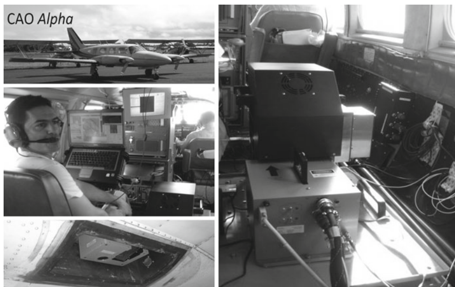
Fig. 18.3 The Carnegie Airborne Observatory (CAO) Alpha sensor package flew from 2006 to 2011 on a variety of aircraft, such as the Piper Navajo shown in the upper left panel . The Alpha system included a Visible-to-Near-Infrared (VNIR) imaging spectrometer and a waveform light detection and ranging (LiDAR) scanner ( right and bottom left panels ). The system was operated using computers and high-performance navigation equipment ( left center panel )
