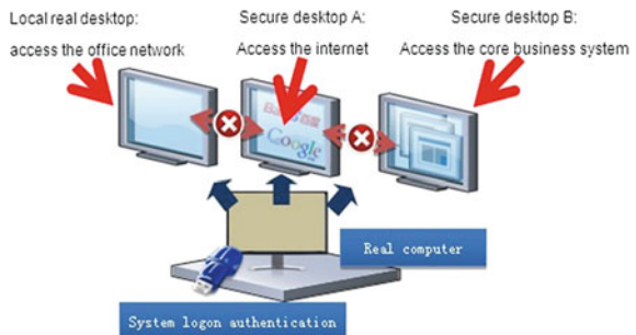
Fig. 90.1 The application model of the secure desktop in the internal network security management
