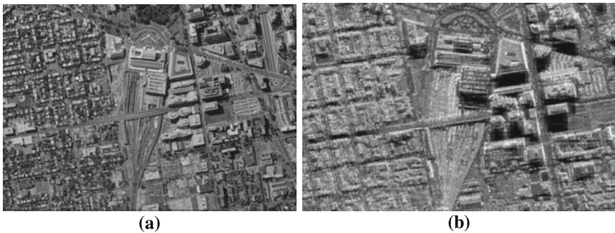
Fig. 55.2 Original optical-SAR image pair. a Optical image. b SAR image
