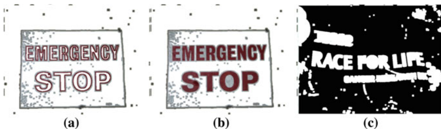
Fig. 57.2 a Not use LCRA; b use LCRA; c result of test image after this step processing
