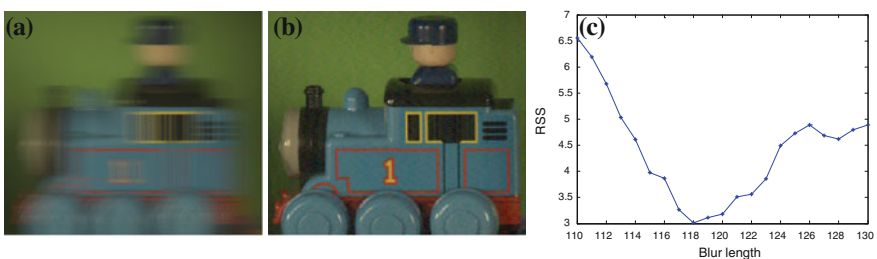
Fig. 52.4 Validity check of our method with Raskar's image. a Coded exposure image supplied by Raskar. b The deblurred image with correct blur length. c The RSS of deblurred images for different estimated blur length
