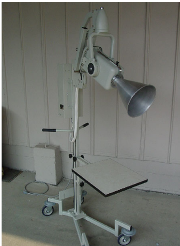
Fig. 3 Portable grenz ray unit by X-Cel X-Ray Corporation
