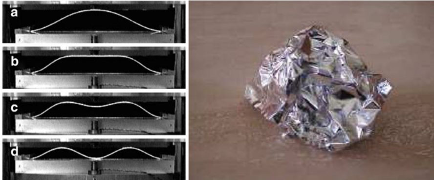
Fig. 7.3 Left : buckling cascade on a sheet compressed between parallel plates [18]. Right : crumpled paper crushed in hands
